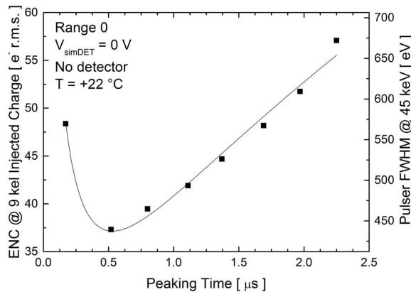
Fig. 3. Intrinsic noise of the readout ASIC measured at room temperature as function of the processing peaking time.
