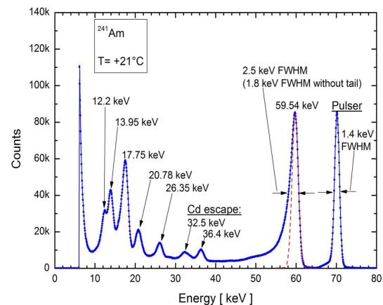
Fig. 5. Energy spectrum obtained with an uncollimated <sup>241</sup>Am source at +21°C. A linewidth of 2.5 keV FWHM @ 59.54 keV is measured. The pulser width is 1.4 keV FWHM.
