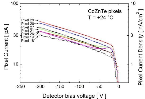
Fig. 4. Pixel dark current density as a function of detector bias voltage. The dark current is always lower than 5nA per square centimeter at 200 V (detector operating voltage).
