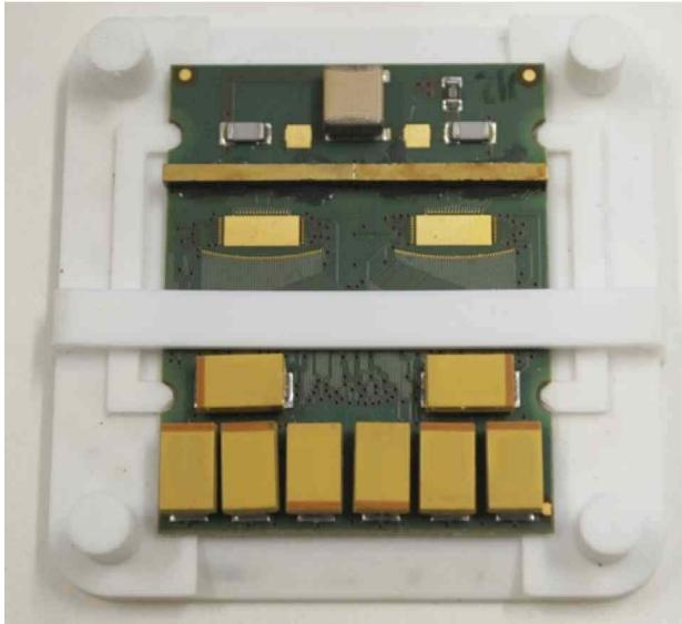
Fig. 2. 32 pixels array detector bonded on PCB with housing for ASICs.
